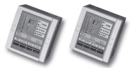
Display modules provide real-time indication of the status of an Xtralis VESDA detector. They have a 20-segment vertical bar graph display, a 2 digit numeric display, an audible sounder, clear alarm and fault indicators. They also have 4 push button keys to control the detector and the mode of the display.
